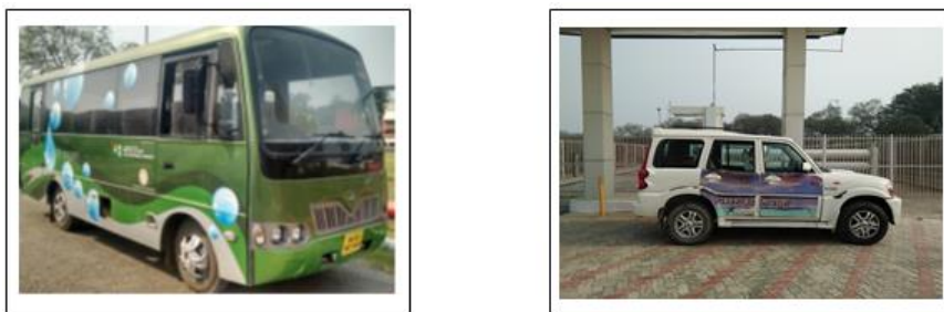
Figure 2.13: HICE Mini Bus and Hydrogen-Diesel Dual Fuel Vehicle developed by M&M
