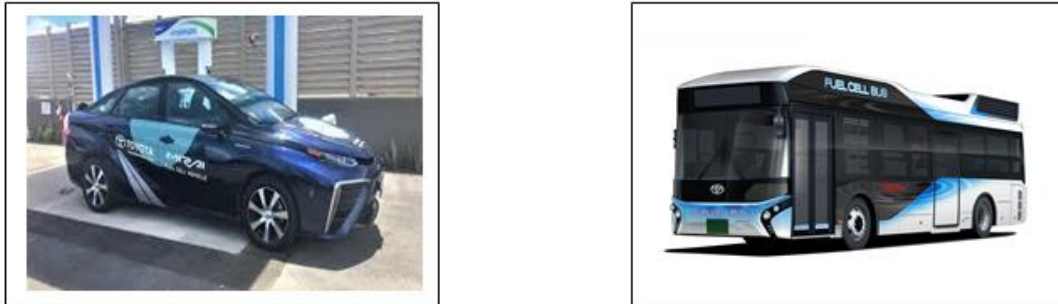
Fig. 2.9: 'Mirai' – A fuel cell Car and 'Sora' - A fuel cell bus developed by Toyota
