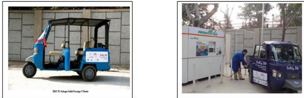
Fig. 2.11: Hydrogen Fuelled ICE Three-Wheelers developed by IIT Delhi and M&M
