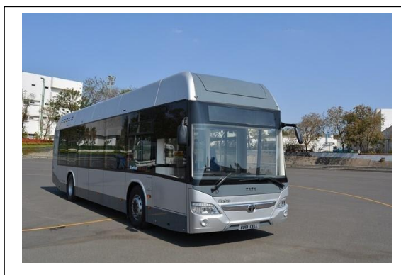
Fig. 2.14: Fuel Cell Bus developed by Tata Motors
