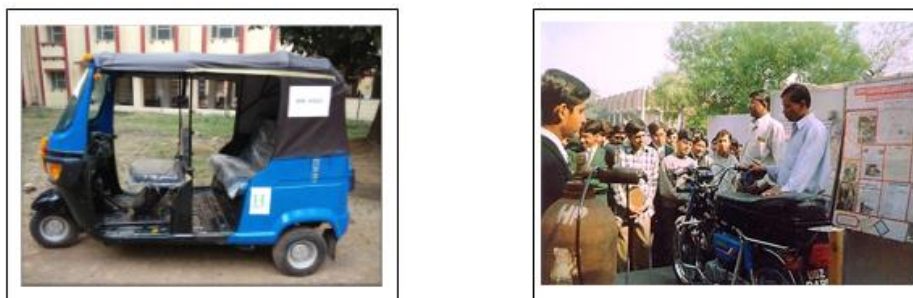
Fig. 2.12: Hydrogen fuelled three-wheeler and Motor-cycle developed by BHU, Varanasi
